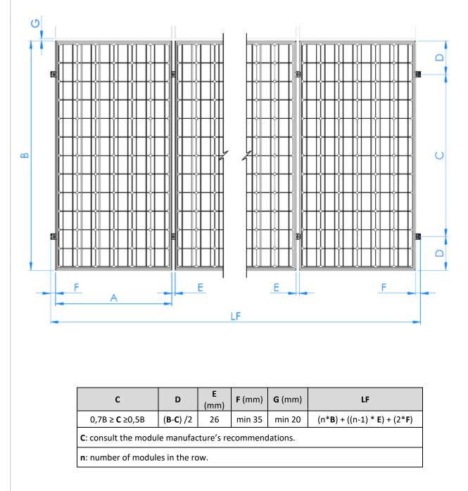
The type of fixing system and the location of its installation points shall be adapted to the needs of the supporting structures and the same time to the needs of the roofs where they must be installed.
