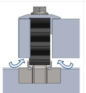
**3.** Insert the corresponding elements, two panels in the case of an intermediate clamp, or a panel and gauge in the case of lateral clamp.
