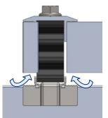
**3.** Insert the corresponding elements, two panels in the case of an intermediate clamp, or a panel and a gauge in the case of a lateral clamp.
