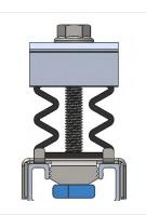
1. Place the clamp in the profile with the lower nut parallel to the profile.
